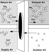
wheels using 3Å/4Å (mole-cular sieve) mixtures as the desiccant; however would allow even the smallest diameter pollutants to blow over, because the pore size of the desiccant will essentially allow molecules smaller than 3Å in diameter, 5000 times smaller than the diameter of the human hair to pass into the fresh air supplies. Water molecules, 2.8Å in diameter, can enter and exit the sieve. As a result, the contaminations remain in the exhaust air stream.
