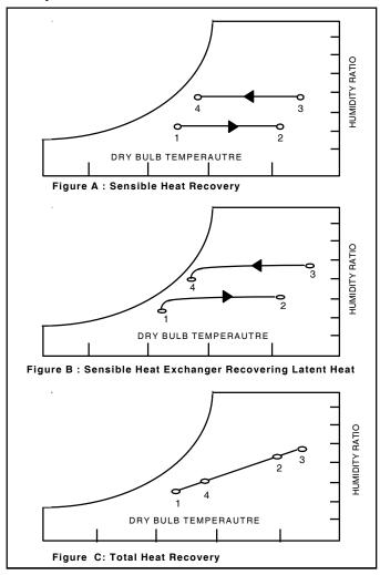
Figure B illustrates a sensible process in which condensation occurs in the hot air stream along with evaporation in the cold one. In this case, latent heat transfer enhances the overall wheel effectiveness. Figure C depicts the total heat recovery process of the enthalpy wheel, assuming mass flow rates in the air streams are the same, and latent and total heat effectiveness are equal.
